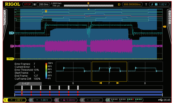
▲ Fig. 4 Using 4000 series scope capture reveals a glitch in the center of the mask, captured in a recording of frames.
